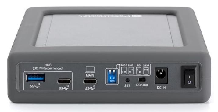
My goal is not redundancy but mostly a large SSD-based storage media. So I decided to use RAID-0 to have max performance with two 8TB Samsung SSDs.
